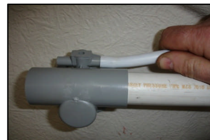
Push 19mm flex pipe on barb spigot.
