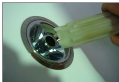
Using Installation tool MT0168 rotate in clockwise direction, a clipping action indicates jet is locked in place
