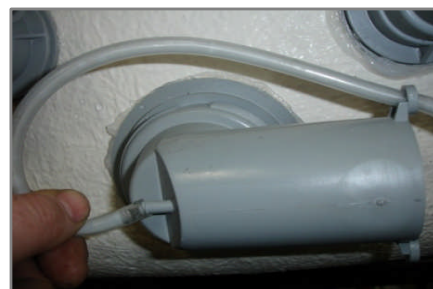
Glue and fit 5mm ID tube as shown feeding through retaining lugs to prevent accidental removal.
